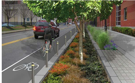
Figure 8: Low Impact Development Stormwater Management Techniques Incorporated into Street Design. This sort of design is encouraged in the McCormick Village Subarea.
